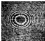
Figure 1 : Interference rings monitored with a 0.4 \text{cm}^{-1} free spectral range Fabry-Pérot. The OPO emission linewidth can be estimated to 0.08 \text{cm}^{-1} .
