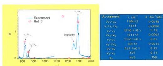
Absorption spectrum of gas mixture under investigation and observed spectral features identification.
