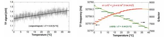
Fig. 3. Temperature dependence of the QEPAS signal (0.7 s data acquisition time) for 100ppm  $C_2H_4$  (a) and of the TF *Q*-factor and resonance frequency (b).
