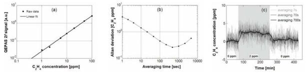
Fig. 2. (a) Sensor response to varying  $C_2H_4$  concentration; (b) Allan plot for a 13-hour measurement of the sensor zero level; (c) 0-2 ppm  $C_2H_4$  step observed with longer averaging times.
