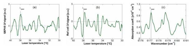
Fig. 1. (a) 2*f* wavelength modulation QEPAS spectrum measured for 100ppm  $C_2H_4$ ; (b) 3*f* signal from the reference cell; (c) comparative  $C_2H_4$ FTIR spectrum (scaled to 100 ppm) from the PNNL database [4]. The selected  $C_2H_4$  absorption peak is indicated by  $\lambda_{peak}$  in each plot.
