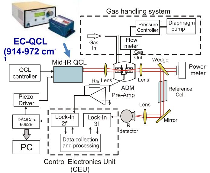
Fig. 2. Real-time breath sensor architecture for ammonia detection.
