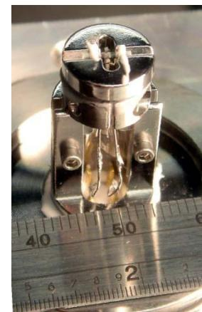
Fig. 1. Quartz tuning fork based spectrophone with acoustic resonator for signal to noise ratio enhancement.
