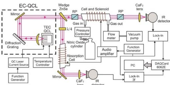
Fig. 3. External Cavity Quantum Cascade Laser based Faraday Rotation Spectrometer for nitric oxide detection.
