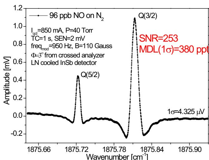
Fig. 4. Faraday rotation spectrum of  $Q_{3/2}(3/2)$  and  $Q_{3/2}(5/2)$  transitions of NO centered at  $1875.8 \text{ cm}^{-1}$  measured for a 96 ppbv in  $\text{N}_2$  mixture at 40 Torr. Using liquid nitrogen cooled InSb photodetector. The analyzer angle is  $3^\circ$ , the time constant is 1 second and the modulation is 110 G at 950 Hz.
