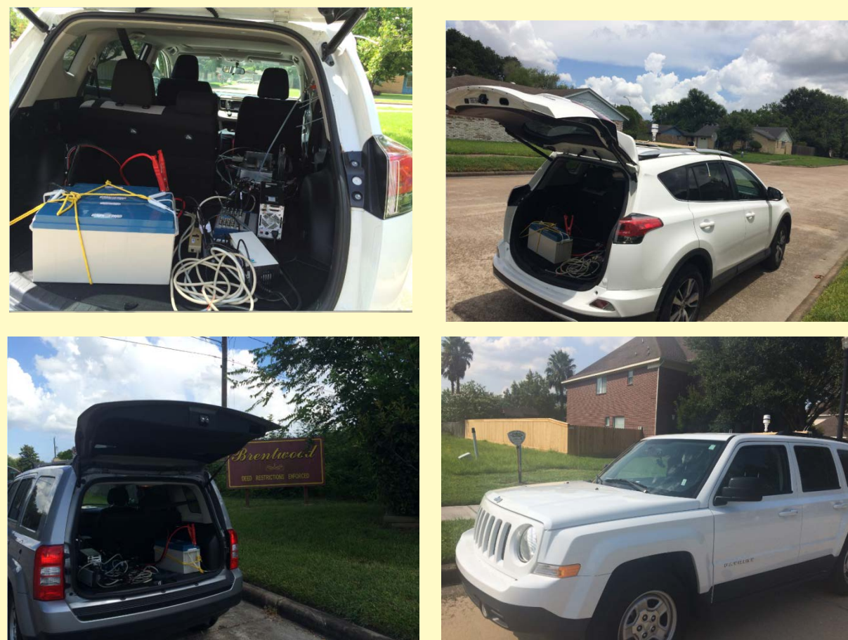
Fig. 6 Sensor unit with weather station, power supply, pressure and temperature control systems deployed in a vehicle at different locations in the Houston area during summer 2016
