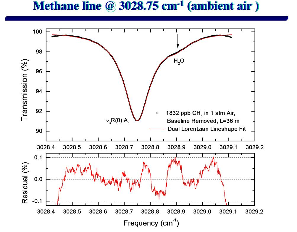
Methane concentration measurement in ambient air
