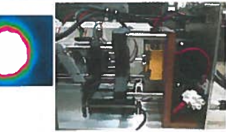
CW HHL TEC DFB-QCL package and IR camera image of the laser beam at 630 mA and 20.5 deg C through tubes after ADM
