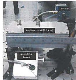
Innovative long path, small volume multipass gas cell: 57.6m with 459 passes
