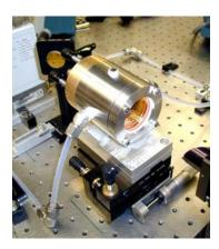
The optimum NO detection sensitivity at 1920.7 cm<sup>-1</sup> realized to date is 15 ppb.
