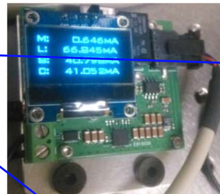
Laser current driver with dimensions of 4.2 × 4.8 × 2.0 cm 3
