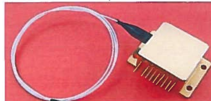
A. Lyakh, et al "1.6 W high wall plug efficiency, continuous-wave room temperature quantum cascade laser emitting at 4.6 \mu\text{m} ", Appl. Phys. Lett. 92, 111110 (2008)
