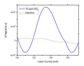
Fig. 2: 2f sensor signal for moisturized 10 ppm mixture of SO<sub>2</sub> and N<sub>2</sub>(blue plot), dotted curve represents optical sensor baseline. Total gas pressure for scan was 200 Torr
