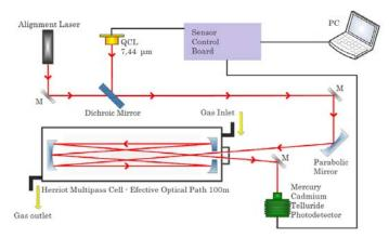
Fig. 1: Schematic of SO<sub>2</sub> gas sensor using a 7.44 µm DFB -QCL as the excitation source, M- mirror
