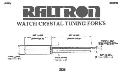
Frequency: 32.768kHz ±30ppm. Operating temperature: -10°C to +60°C
