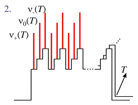
Fast cycling of the laser frequency with a subthreshold current and slow scanning with temperature (wavelength modulation)
