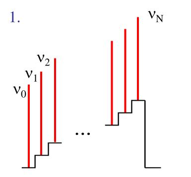
Synchronous digitally synthesized steps of tuning current (enables linearization of scan)
