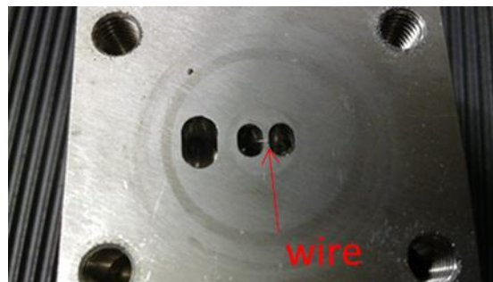
Figure 2. Photograph of the internal part of a vacuum valve. In the picture a small wire inserted between two holes to simulate a leak is visible.
