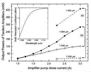
Fig. 2. Amplifier output powers as a function of the 3-W (at 3 A) pump diode current. (a) Pump wavelengths of 1064 and 1550 nm with seed powers of 40 and 10 mW, respectively (b). Pump wavelengths of 1083 and 1550 nm with seed powers of 20 and 10 mW, respectively. Inset, measured absorption coefficient of Er/Yb fiber as a function of wavelength.
