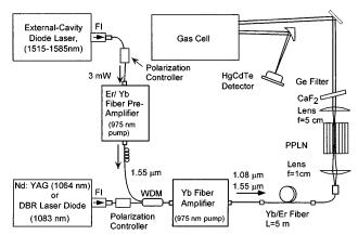
Fig. 1. Schematic of the dual-wavelength amplifier—pumped DFG source—based gas sensor: FI's, Faraday isolators.
