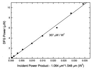
Fig. 3. DFG power at 3.4  $\mu m$  versus pump power mixing product  $P_{1064 \text{ nm}} \times P_{1550 \text{ nm}}$  for a 2-cm PPLN crystal.
