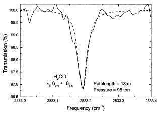
Fig. 5. Absorption spectrum of the  $\nu_5$   $6_{0,6} \leftarrow 6_{1,5}$  transition at 2833.2 cm $^{-1}$  for a calibrated 5.78-ppm  $H_2CO$ -in- $N_2$  mixture. A Hitran 96 spectrum of 5.78-ppm  $H_2CO$  is shown for comparison.
