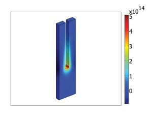
FIG. 14. The first principal stress (Pa) of the 32.8 kHz QTF at the resonance frequency.
