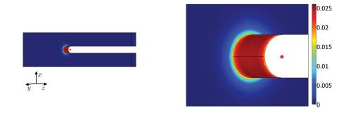
FIG. 4. Left: The numerical solution of the amplitude of the thermal wave on the surface of the QTF. Right: Zoomed in plot where the temperature is largest. For this simulation, the laser source was centered at  $(x_s, z_s) = (0, 0)$ . (The red dot shows the intersection of the laser beam axis with the xz-plane.)
