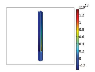
FIG. 16. The first principal stress (Pa) of the 3 kHz QTF at the resonance frequency.
