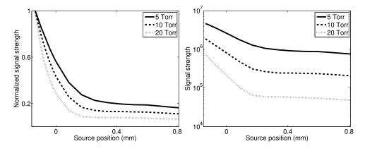
FIG. 10. The normalized amplitude of the ROTADE signal obtained from numerical simulations as a function of laser positions on a linear scale (left) and a log scale (right). These results are for  $CO_2$  at three ambient pressures: 5, 10, and 20 Torr shown with solid, dashed, and dotted lines, respectively. The magnitude of the slope of the amplitude decreases as we decrease the ambient pressure.
