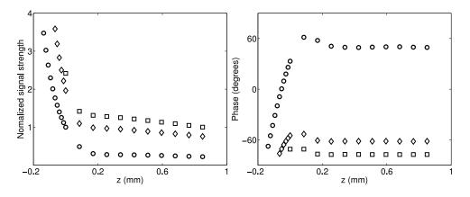
FIG. 8. Amplitude (left) and phase (right) of the piezoelectric current as functions of the vertical position of the laser beam. The results shown with circles, diamonds, and squares correspond to the laser source positions shown using the same markers in Figure 7.
