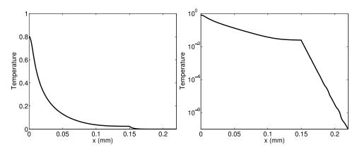
FIG. 5. One-dimensional slice of the temperature distribution computed in the exterior (0 < x < 0.15 mm) and interior (x > 0.15 mm) of the QTF. The slice is taken at (y, z) = (0, 0) and along the x-axis. For this simulation, the laser source was centered at  $(x_s, z_s) = (0, 0)$ , and the thermal source,  $S_T$ , was normalized to have value 1 at (0, 0, 0). The right figure is a semilog plot of the temperature shown in the left figure.
