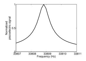
FIG. 6. The magnitude of the piezoelectric current as a function of frequency.
