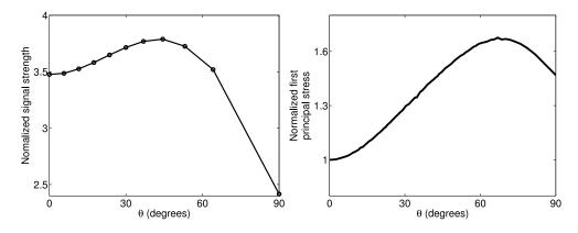
FIG. 9. Left: The amplitude of the piezoelectric current as a function of the angle from the negative vertical axis of the QTF. The laser source positions were chosen to lie on a circle of radius 0.0137 mm centered at the origin. Right: The first principal stress of the QTF as a function of the angle around a circle located between the tines of the QTF and at a distance of 0.02 mm from the inner surface.
