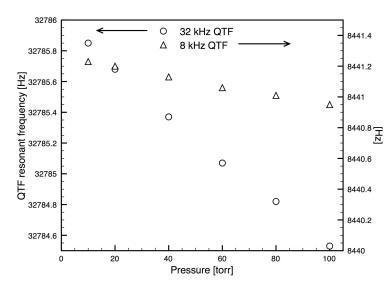
Figure 2. QTF resonant frequency at various pressures.
