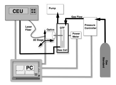
Figure 1. Experimental Setup. The DFB fiber-coupled diode laser was modulated at  $f_0/2$  of the QTF, the computer controlled 3D stage had a resolution of  $1\mu$ m, and the beam had a waist size of approx. 15  $\mu$ m.
