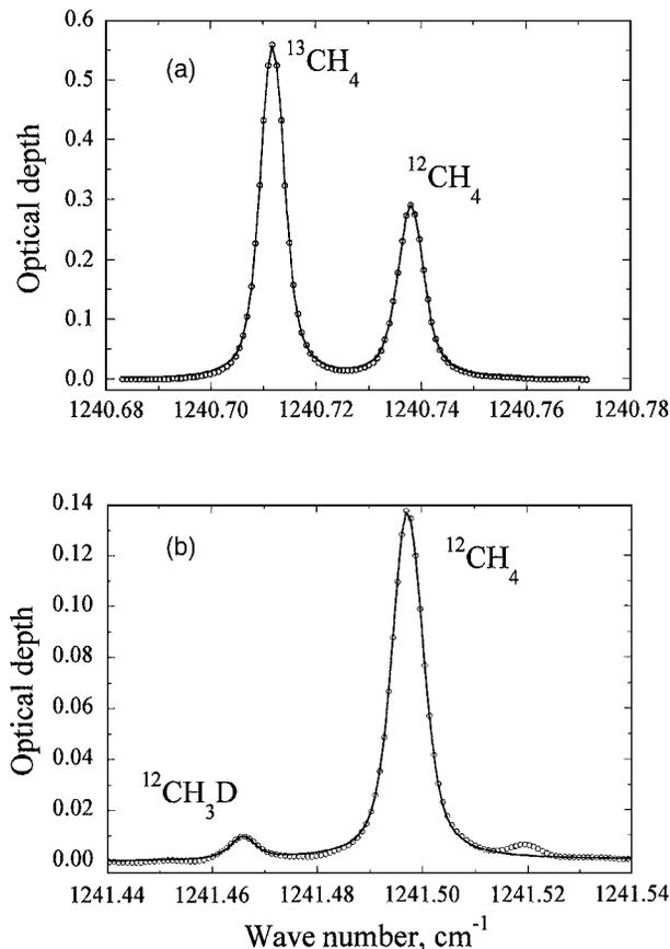
Fig. 4. (a) Absorption lines used to define the  $^{13}\text{C}$  content in the  $\text{CH}_4$  sample. (b) Absorption line of the deuterated  $\text{CH}_4$ . The open circles represent the measured data, and the solid curves represent their Voigt fitting.
