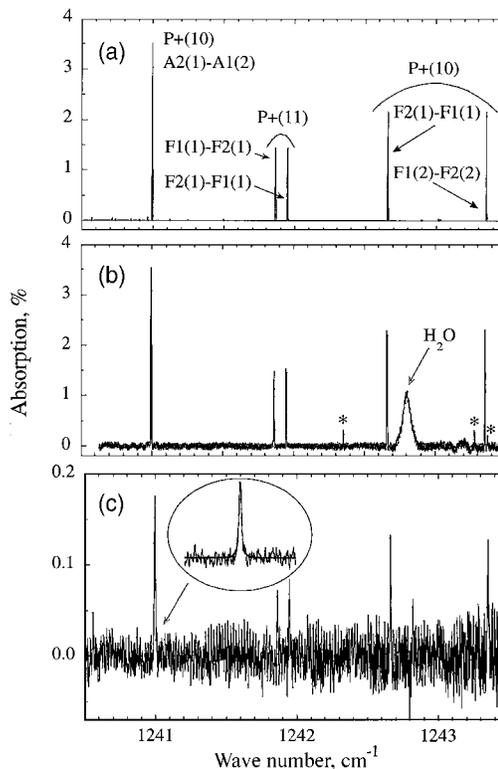
Fig. 3. (a) Simulated absorption spectrum of CH<sub>4</sub> (6.5 mTorr, 43 cm) and (b) measured spectrum for the same conditions. The false absorption lines that appear because of the two-mode lasing are marked with asterisks. (c) Measured spectrum of 20 ppm of CH<sub>4</sub> in 50 Torr of air. Inset, the Voigt fit of the strongest absorption line. The path length is 43 cm for all three spectra.
