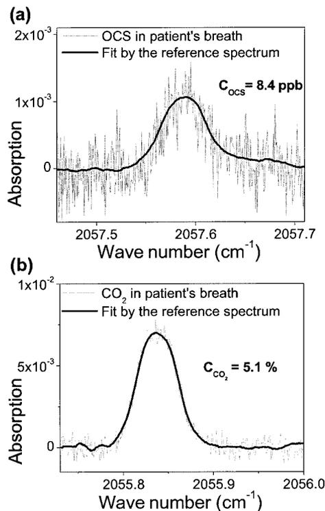
Fig. 8. Measured spectra and calculated concentrations of (a) OCS and (b)  $\text{CO}_2$  in a breath sample of a lung transplant recipient. [The baseline was fitted in the frequency range on each side of the absorption line and subtracted to create plot (a)].
