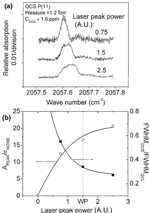
Fig. 3. (a) Relative absorption in a low-pressure (1.2-Torr) OCS sample as a function of wavelength depicting the QCL linewidth for three different optical power levels. (b) Spectral SNR,  $A_{\text{PEAK}}/\sigma_{\text{NOISE}}$ , and sensor selectivity  $\text{FWHM}_{\text{OCS}}/\text{FWHM}_{\text{QCL}}$  versus laser peak power. WP, working point chosen for experimental measurements.
