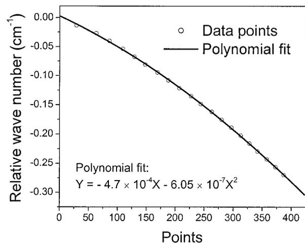
Fig. 5. Calibration curve of the QCL frequency scan.
