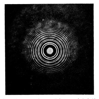
Fig. 4. Interferogram of quartz optical resonator obtained with He–Ne laser illumination. Two axial modes (mode separation  $\sim$ 600 MHz) appear well resolved.
