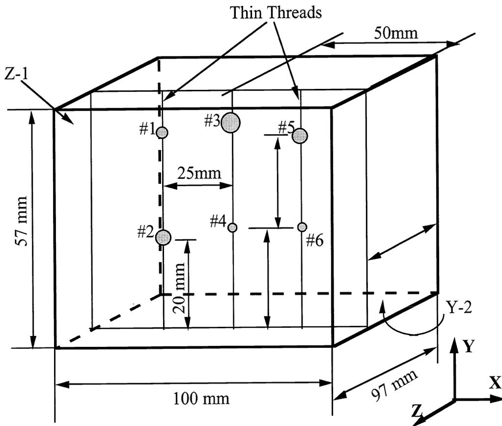
**Figure 3.** 3D schematic diagram of the gelatin breast phantom with absorbing spheres simulating tumors. Diameters: 3, 4, 6, 2, 4, and 2 mm (spheres #1, 2, 3, 4, 5, and 6, respectively).
