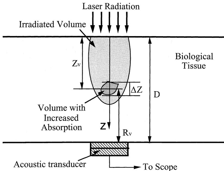
**Figure 1.** Generation and transmission mode detection of optoacoustic pressure waves in tissues.
