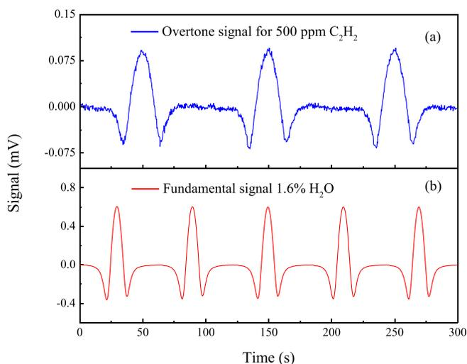
FIG. 5. Simultaneous dual-gas measurements using a QEPAS sensor based on combined vibration motion of a QTF. The optimized modulation depths for  $C_2H_2$  and  $H_2O$  detection were  $0.51\text{ cm}^{-1}$  and  $0.43\text{ cm}^{-1}$ , respectively.
