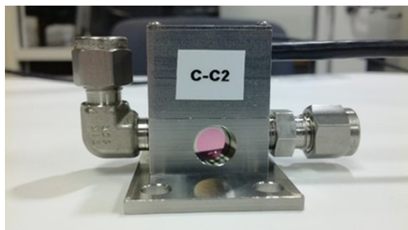
FIG. 2. Photograph of an ADM. An optical window and the gas inlet and outlet connectors are also visible.
